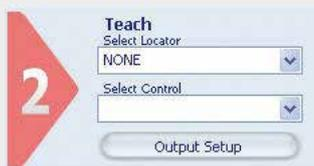
The second step establishes the acceptance criteria to distinguish objects from wastes. One or more controls can be selected according to the task to carry-out.
