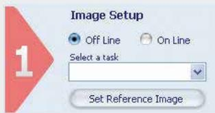
The first step consists in connecting the sensor and configuring the image quality parameters. When the desired results are obtained, the user can memorise the image that will be used as a template during sensor functioning.
