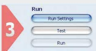
The third step configures the sensor digital outputs, simulates sensor functioning on the PC to verify the controls chosen and activates the operating phase on the sensor using the PC only to control the diagnostics.
