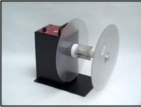
LABELMATE's **Constant Adjustable Torque™ ("CAT")** technology has made the silent, easy-to-use **CAT-3** the "**Industry Standard**" Label Rewinder. There are no awkward troublesome belts or clutches. The **CAT-3-STANDARD** handles labels up to 155 mm (6-inches) wide and will wind a roll of labels up to a 300 mm (12") diameter. Torque and Direction are fully controllable from the Control Panel. Dual torque ranges provide plenty of power for use with a LABELMATE Slitter, too.
