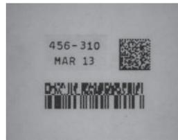
**Glossy label:** Uniformly illuminated resulting in reliable reading and decoding.
