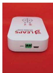
ON/OFF switch allows to switch off the anchor for specific purposes.
