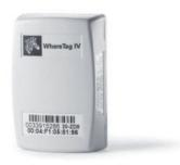
The WhereTag IV enables Zebra Location Solutions to provide fully integrated, "best of breed", Real-Time Locating System (RTLS) solutions. It is compliant with both the ISO/IEC 24730-2 RTLS standard and Cisco Compatible Extensions (CCX) for Asset Tags. Programmable to transmit in either mode or both; operation can be optimized to meet the location requirements of the application.
