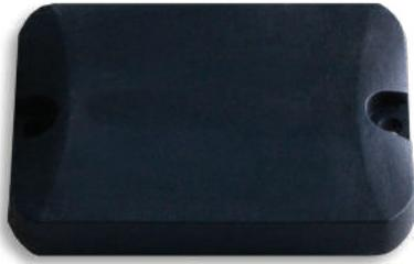
The Xerafy Micro X-II Paintshop is built to perform under extreme heat and repeated exposure to caustic fluids for applications such as hot water wash cycles and post-paint processes. The tag can survive application temperatures of up to 250° Celsius, has an IP68 rating and a read range of up to 10 meters.
